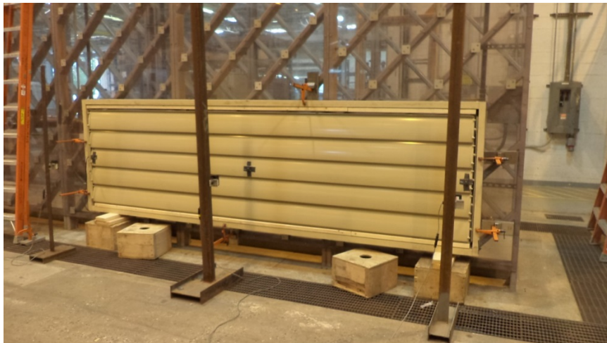
Photo No. 4 14' Unit Set-up for Negative Loads
