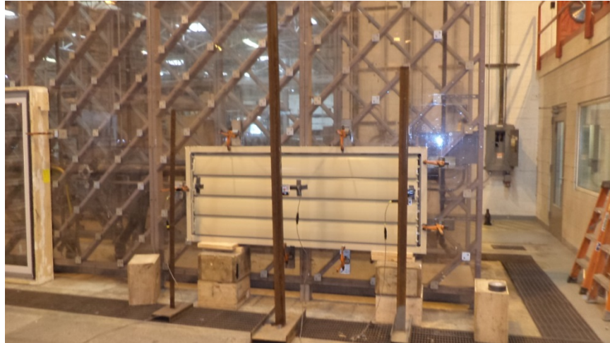
Photo No. 1 8' Unit Set-up for Negative Loads
