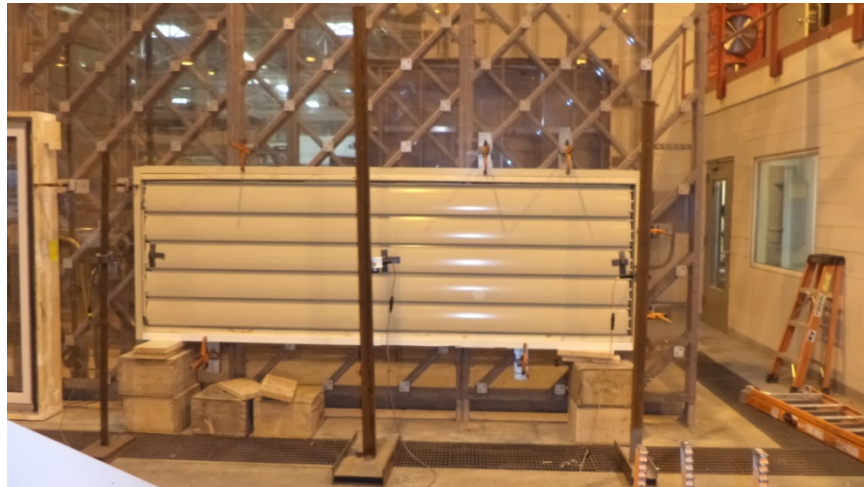
Photo No. 2 12' Unit Set-up for Negative Loads
