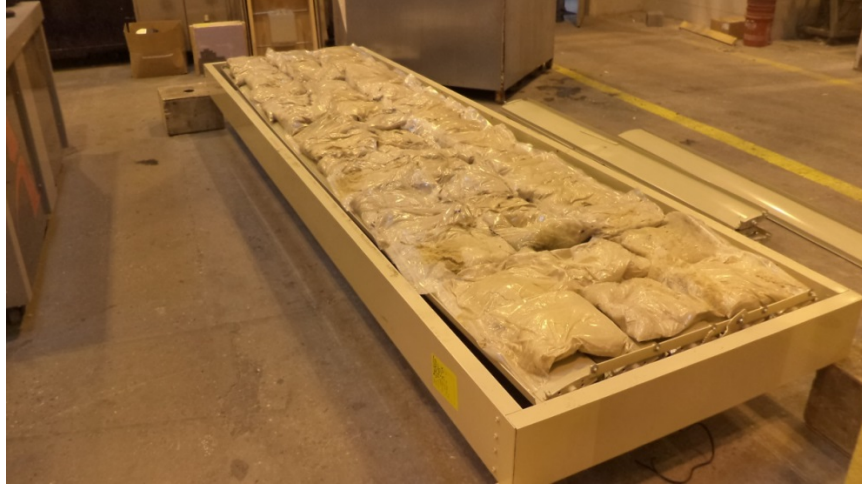
Photo No. 3 14' Unit Set-up for Gravity Load Test
